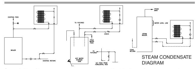
On a typical forced hot water system, connect return to inlet side of circulator and supply upstream of remotely operated valve. Unit may also be connected to mains of an existing loop system of sufficient capacity. Operation will be influenced by the system circulator and associated controls.
